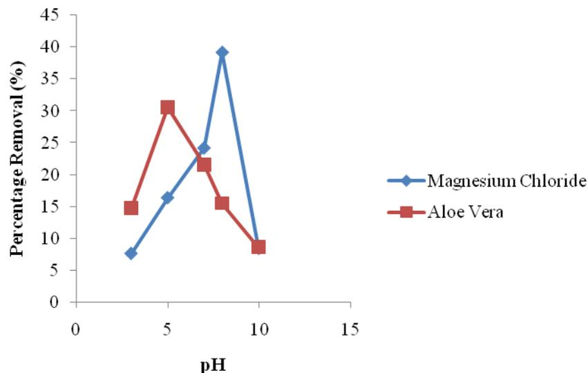
Fig. 3.2: Plot of percentage removal of copper metal ion versus pH.
