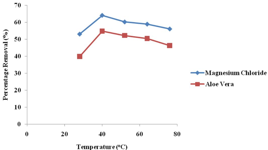
Fig. 3.4: Plot of percentage removal of copper metal ion versus temperature.
