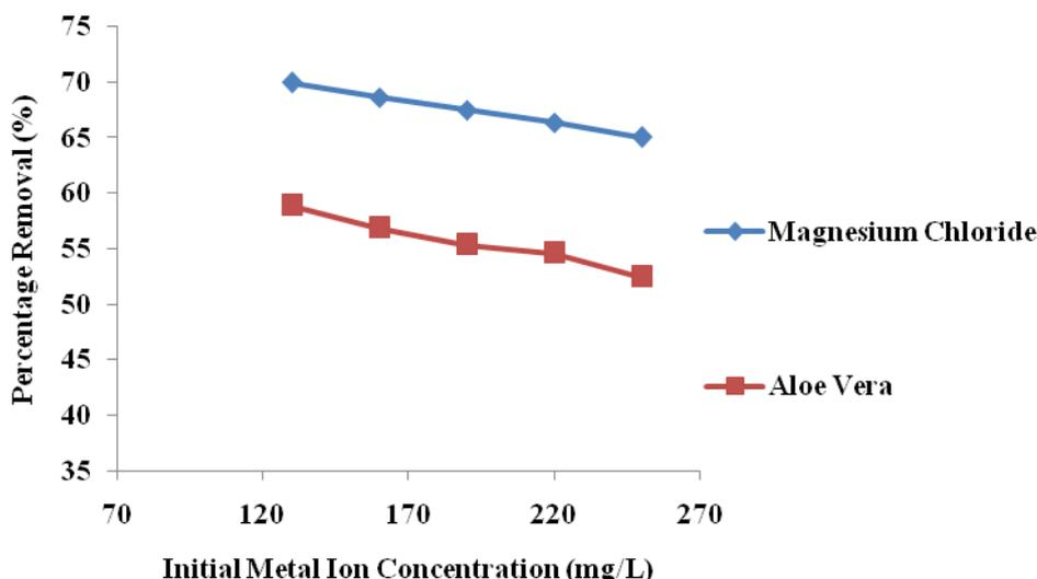
Fig. 3.6: Plot of percentage removal of copper metal ion versus initial metal ion concentration.
