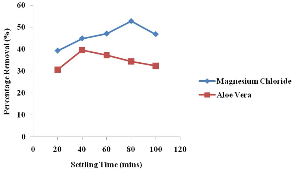
Fig 3.3: Plot of percentage removal of copper metal ion versus settling time.
