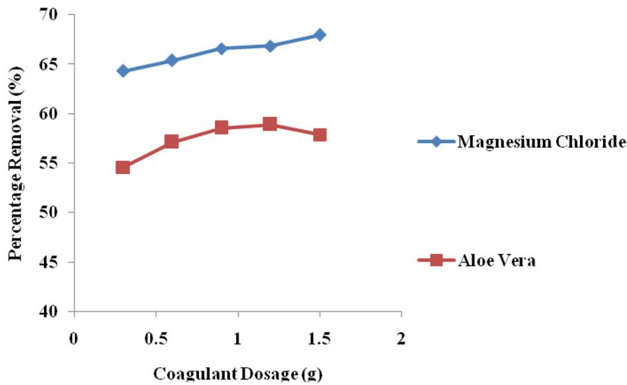
Fig. 3.5: Plot of percentage removal of copper metal ion versus coagulant dosage.
