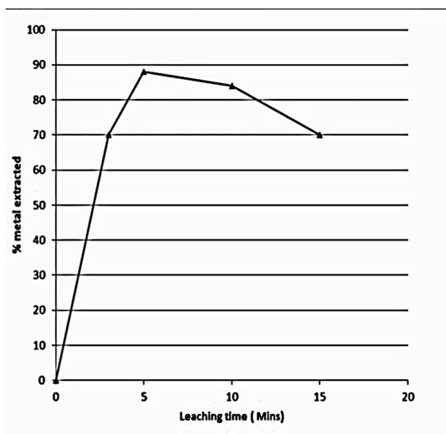
**Figure 3** Plot of leaching of microwave treated cassiterite prior to leaching experiment ( time; 5 mins, particle size, -212  $\mu\text{m}$ ; conc., 4M KOH; Temp., 85° C)
