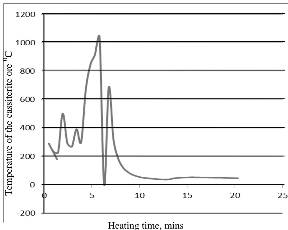
**Figure 1:** Temperature profile of Kuru cassiterite ore at microwave condition of 950W, 2.45 GHz.
