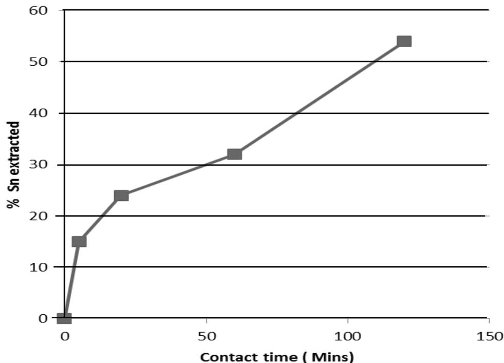
**Figure 2:** Plot of the conventional leaching cassiterite ore. (Experimental conditions: particle size, -212  $\mu\text{m}$ ; agitation speed, 500 rpm; Temperature, 85° C)
