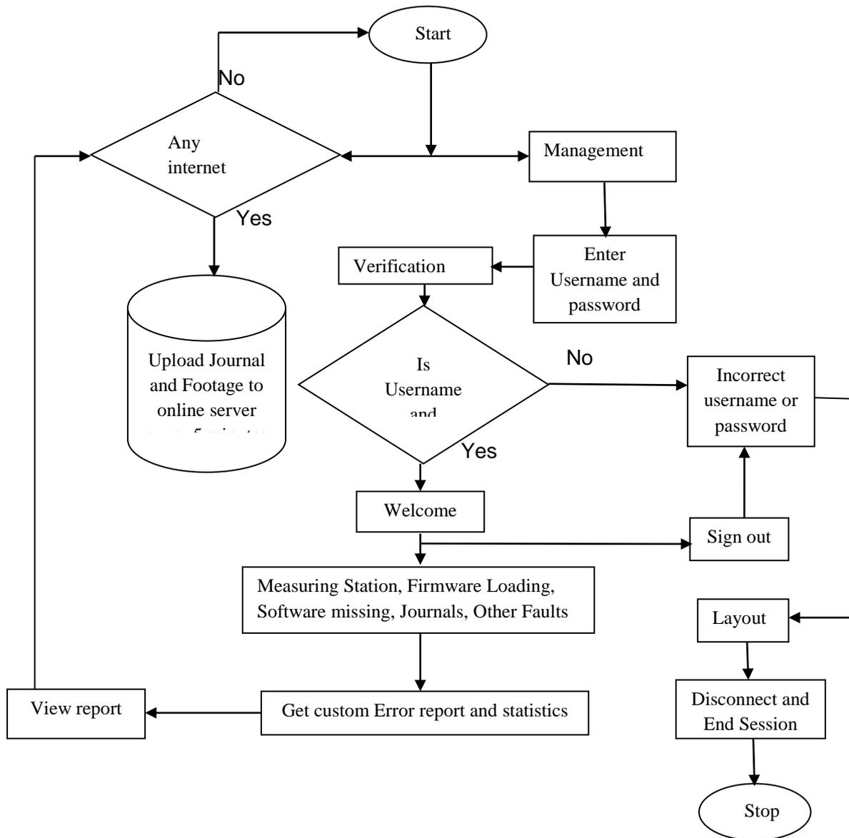
Figure 2: ATM Monitoring Flow Chart for Management
