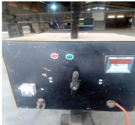
Fig 9: Arc welding machine showing the digital display
