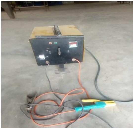
Fig 8: Arc welding machine with casing
