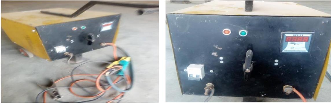
Fig 10: Arc welding machine casing with the handle. Fig 11: Arc welding machine showing the switches.
