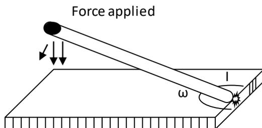
Relating operation in the diagram above to Newton second law of motion, thus torque on a rotating body is directly proportional to the rate of change of angular momentum (Shurne, (2015);
