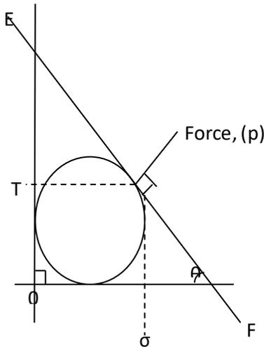
Since the maximum stress  $\sigma_{max} = \sigma_c$  with respect to the shearing stress across the section EF and the maximum shearing stress  $T_{max} = \sigma_c \sin\theta \cos\theta$
