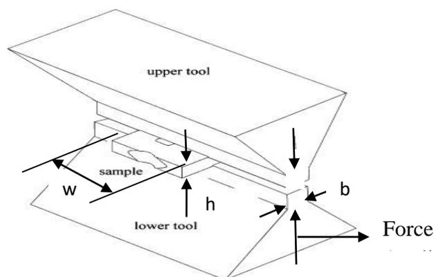
Fig. 1: A schematic diagram of the plane strain compression test set-up (Boldetti *et al.*, 2006).
