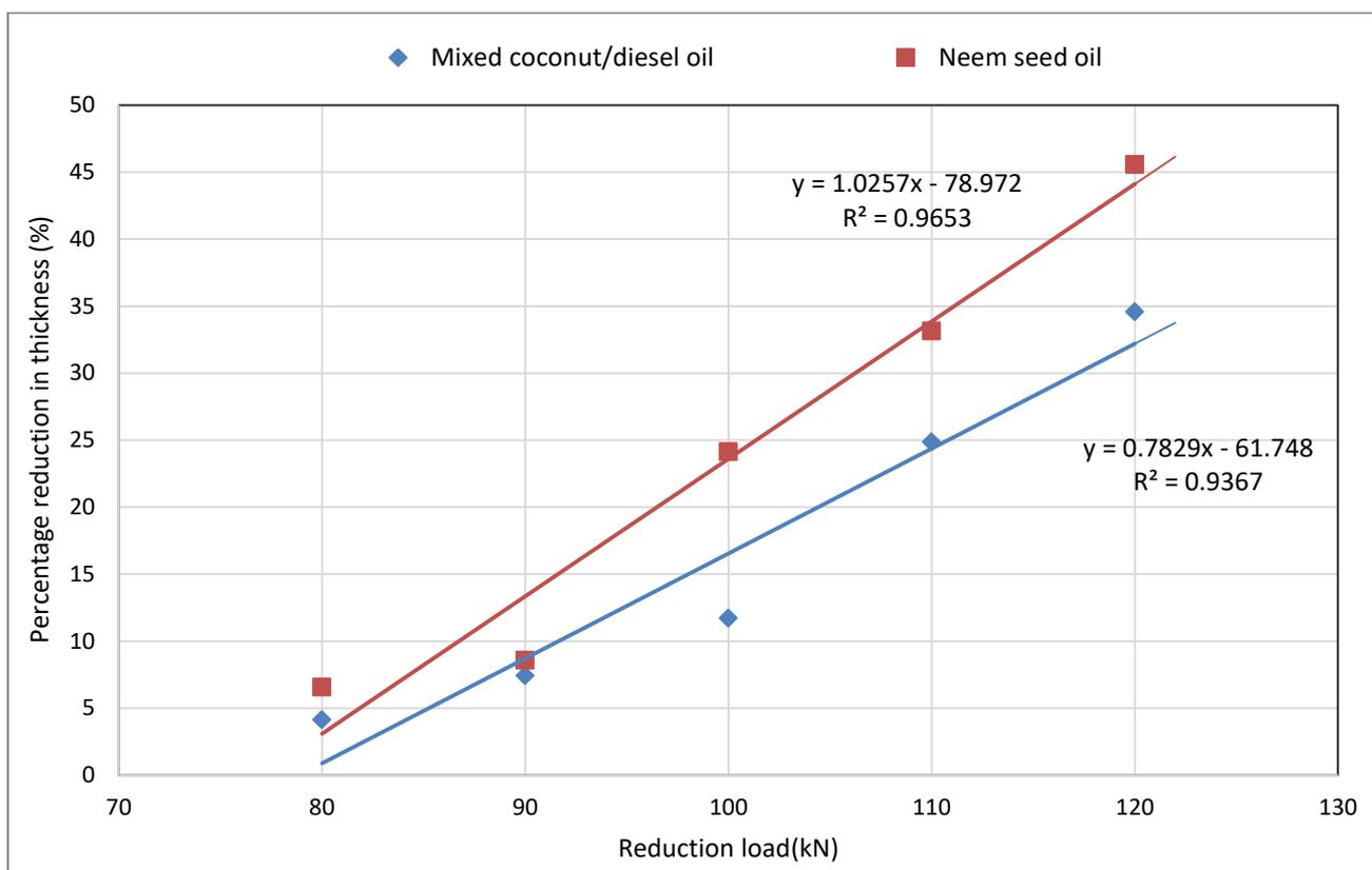
Fig. 2: Reduction capacity of the mixed coconut/diesel and neem seed oils.
