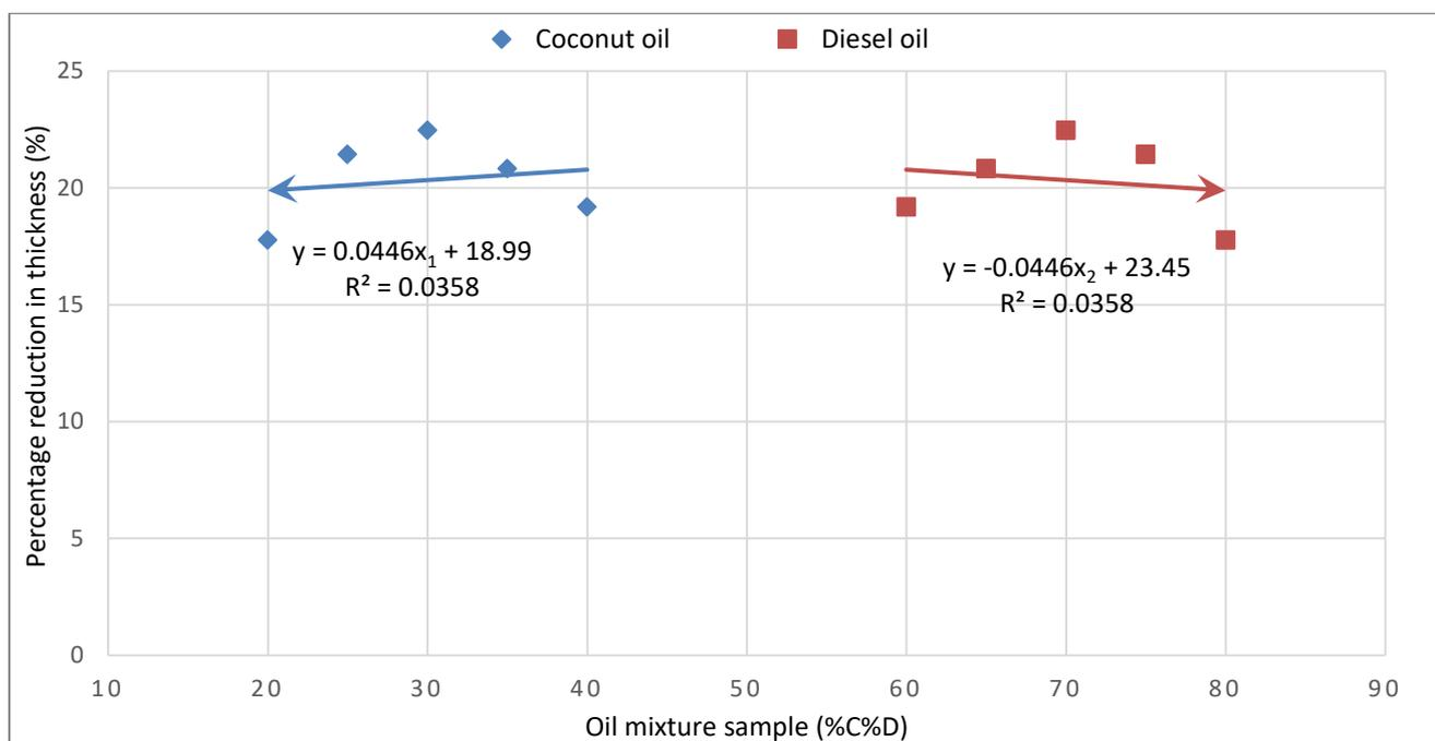
Figure 3: Reduction capacity of the locally sourced coconut oil mixed with diesel in various proportions
