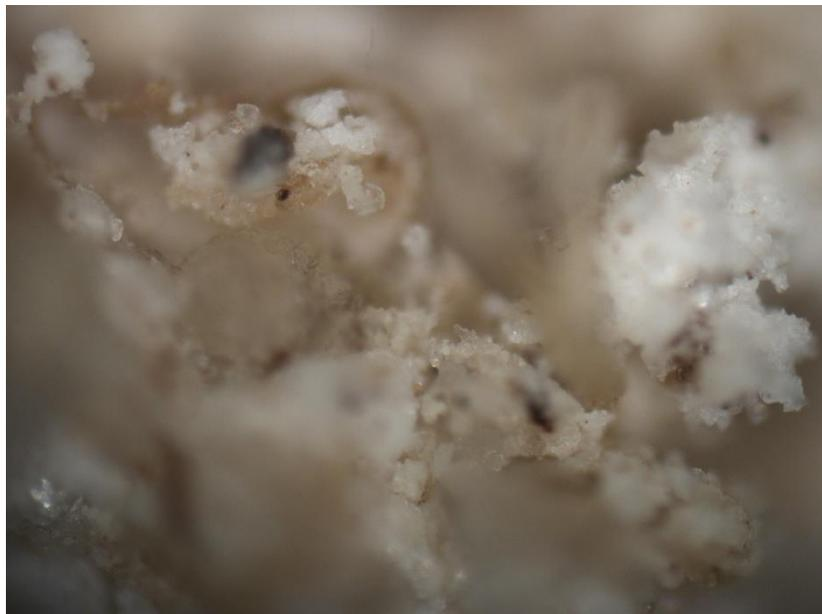
Fig. 5: Microstructure of HDPE reinforced with 25 % coconut shell powder
