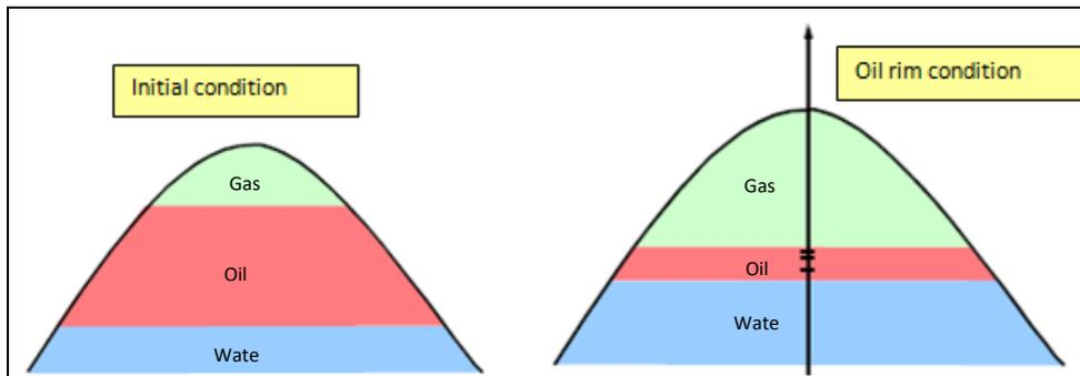
Figure 4: Mature field conditioned as thin oil rim
