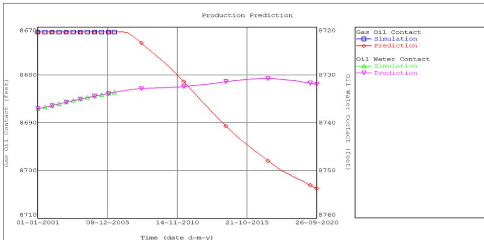
Figure 6: Plot of GOC & OWC vs. Time
